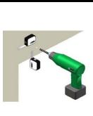
Drill first hole Locate and drill first hole based on BARTELS provided general specification sheets and or project specific Measurement Forms.
